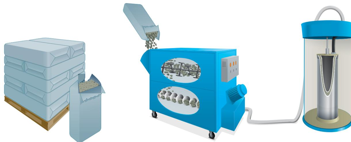
**1** Knauf Insulation CHM S FLOCKS are produced by grinding layers of rock mineral wool into smaller particles. Our production process is fully automated, ensuring **consistent**, premium product **quality**. In order to provide optimal service for our customers different flock sizes are available. **Packaging in compressed bags on pallets** proves a highly efficient storage and transport solution.
